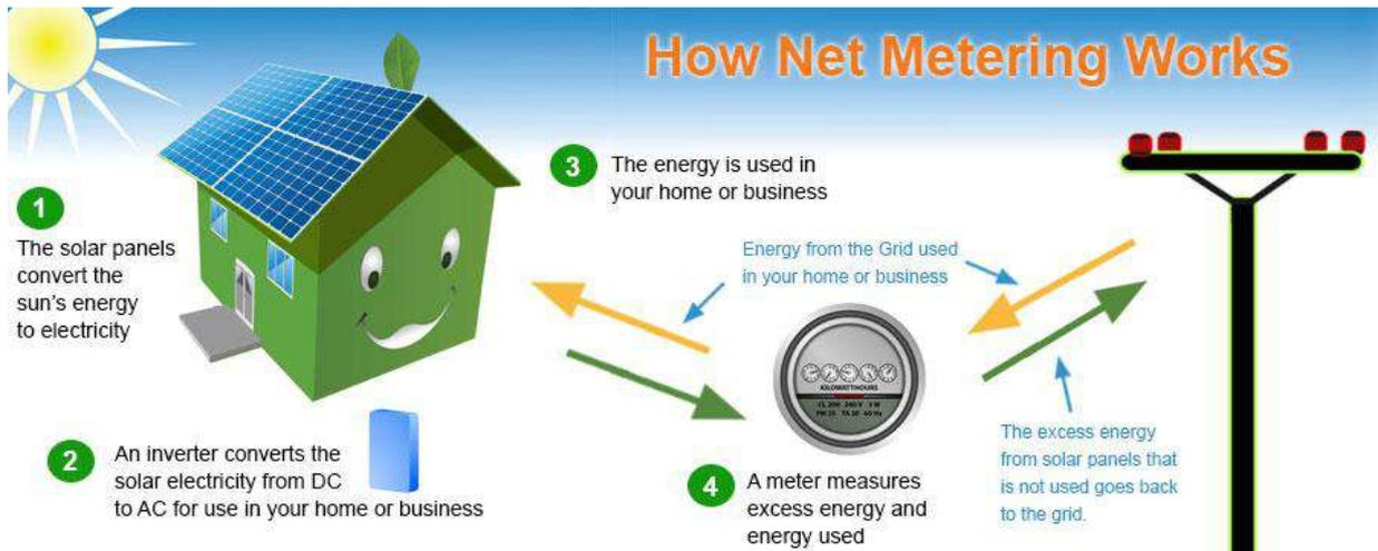
Figure 1.1: Net Metering process
